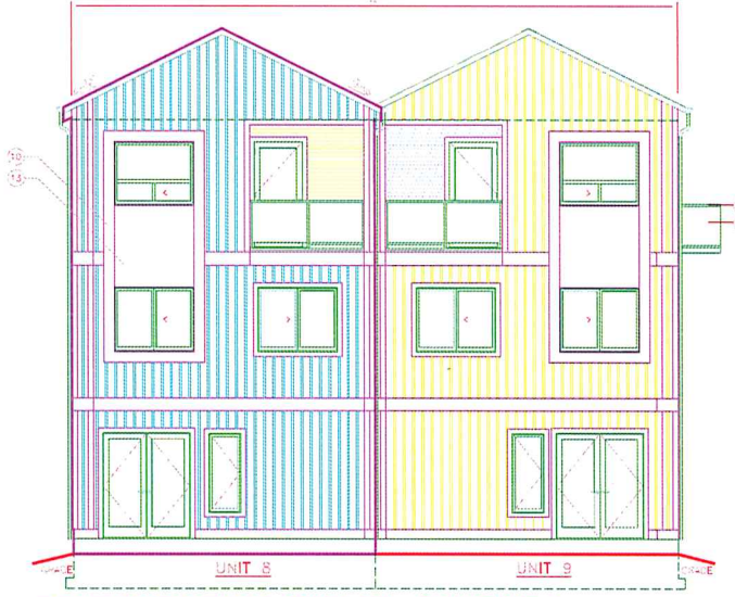
REAR ELEVATION - DUPLEX - BUILDING 3
